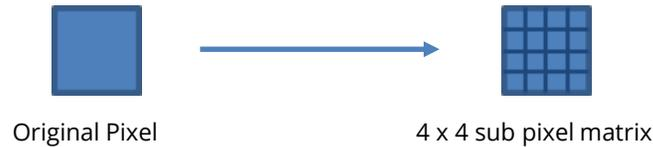
Depending on the original pixel dimensions and the number of sub pixels used, the accuracy of our measurements will be limited to each sub pixel dimension.
